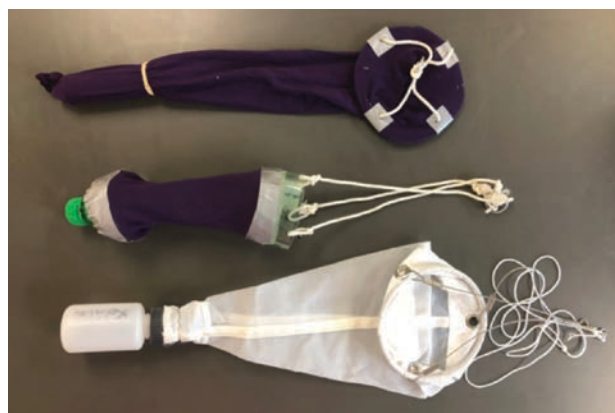
FIGURE 3: Student-constructed plankton nets [top two purple nets] and a commercially available net [bottom white net].
